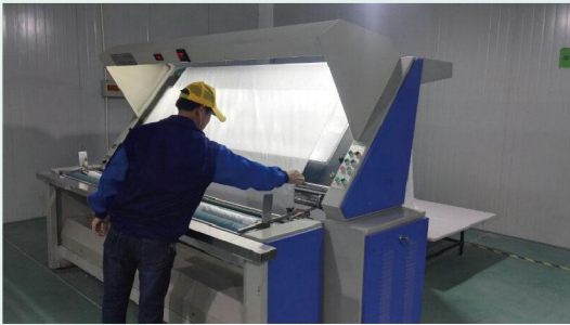
1. Fabric inspection out of warehouse
